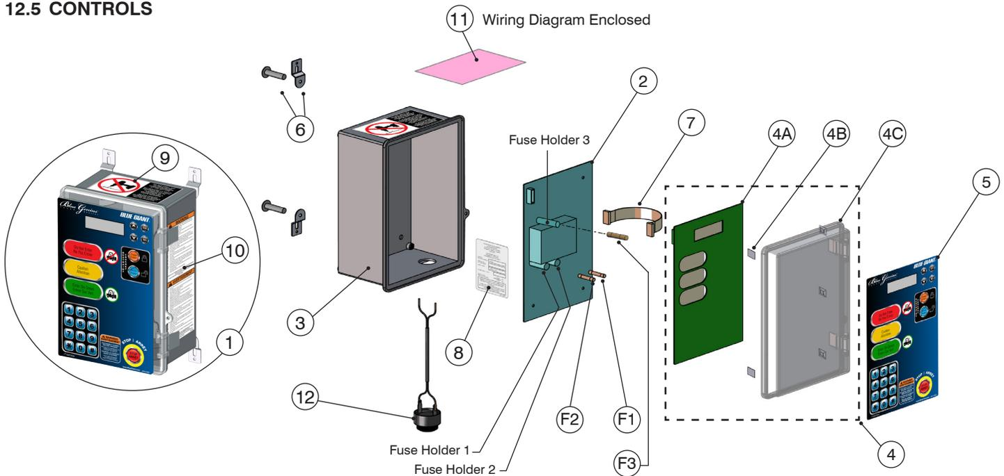
COMPLETE CONTROL STATION ASSEMBLY - ITEM 1 (Example BGG0H1115F)
