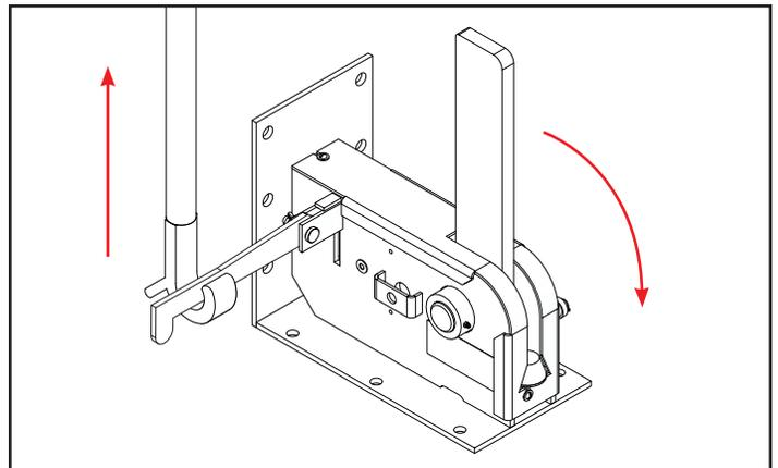
Control rod (part # 782-371) releasing the restraint arm.
