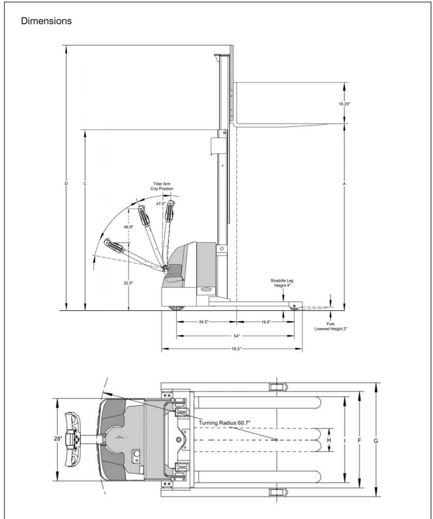
**Note:** Aisle dimensions listed above assume the bay width to be straddled OD plus 2" (1" on either side of straddle leg). Straddled OD is the load width plus 8". \*For metric conversion multiply inches by 25.4.
