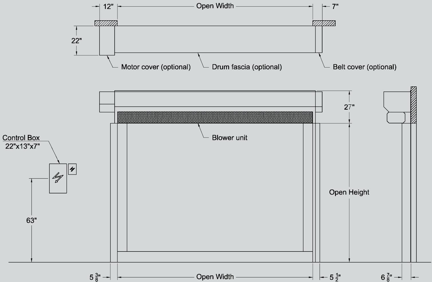
All indicated dimensions are net: the space necessary for mounting and maintenance has to be provided.
