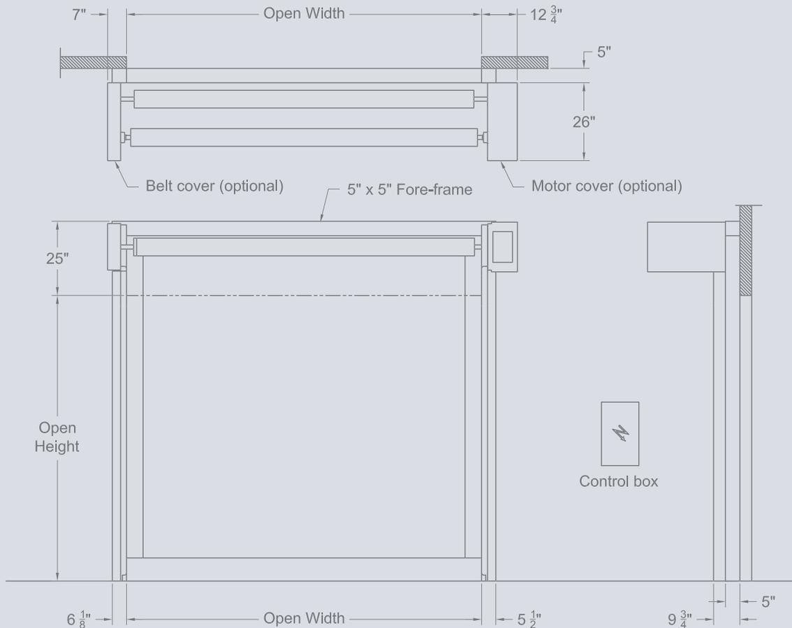
All indicated dimensions are net: the space necessary for mounting and maintenance has to be provided.
