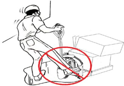
Always look in direction of travel. Keep a clear view, and when load interferes with visibility, travel with load or lifting mechanism trailing except when climbing ramps.
