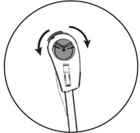
3. Turn the travel switch to move the vehicle forward or backward.
